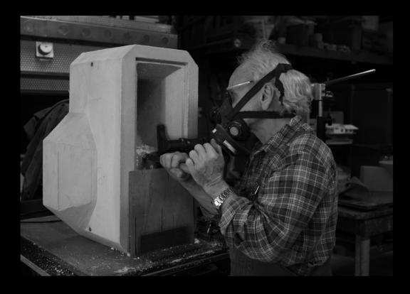
IMAGE / FINAL MOULD READY TO RECEIVE CRYSTAL GLASS
