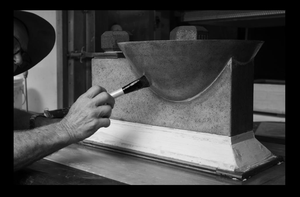
IMAGE / A LAYER OF OIL IS APPLIED OVER SHELLAC TO ASSIST PLUG RELEASE FROM WET PLASTER MOULD
