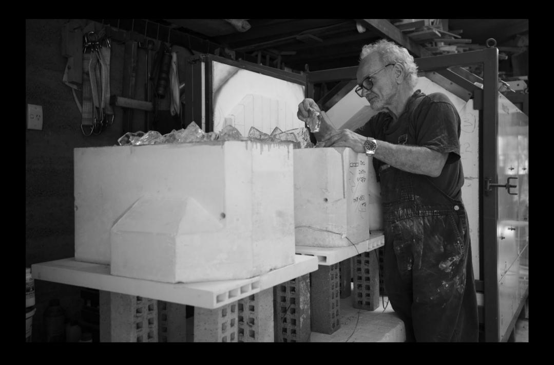
IMAGE / CRYSTAL GLASS IS DELICATELY SELECTED AND ADDED TO MOULDS EDITIONS VESTIGE PROCESS
