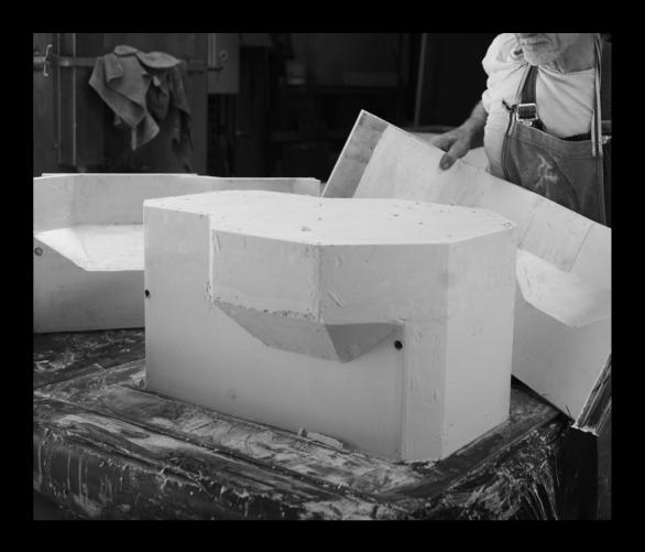
IMAGE / FINAL MOULD STRIPPED AND READY FOR PLUG REMOVAL
