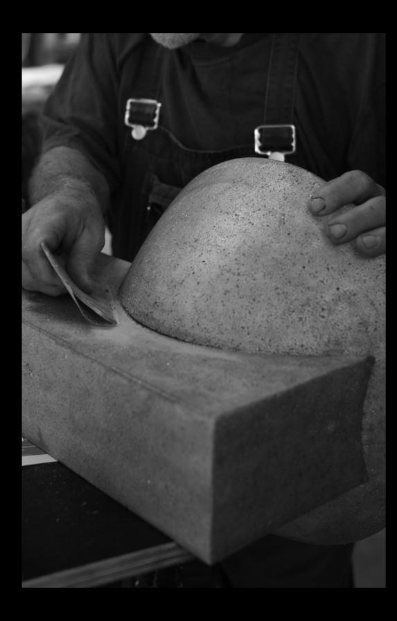
IMAGE / SHELLAC IS ADDED IN LAYERS TO ONE TO ONE PLUG TO SEAL SURFACE
