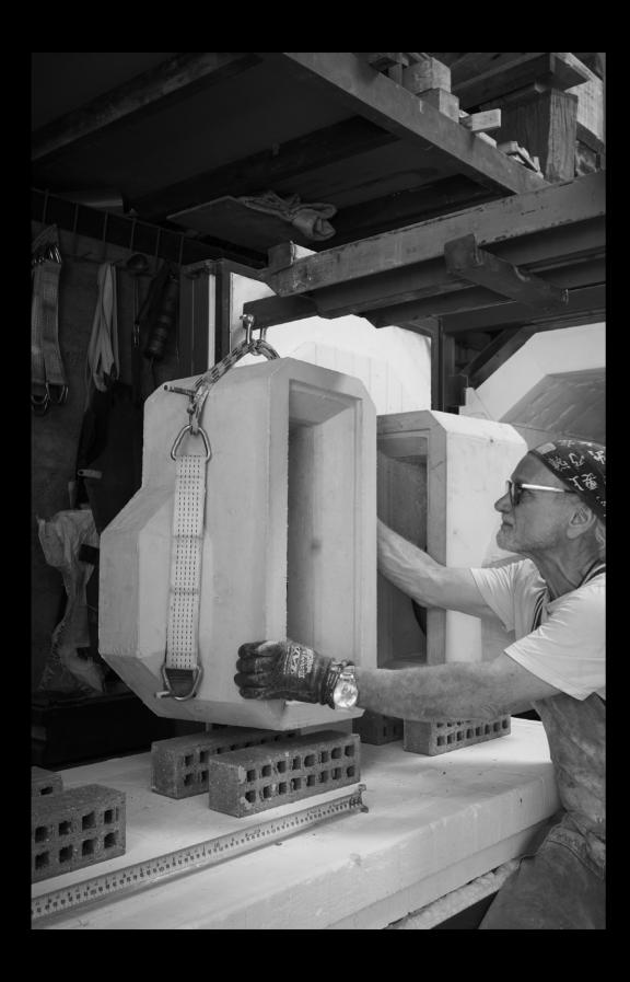
IMAGE / WET MOULDS POSITIONED ON KILN HEARTH TO START PRE DRYING AND CURING
