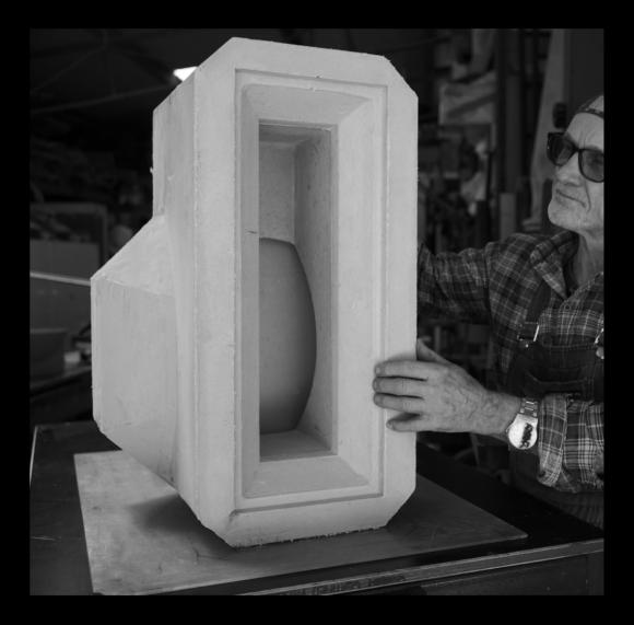
IMAGE / THE INTERNAL PLUG IS REMOVED FROM THE MOULD BY HAND
