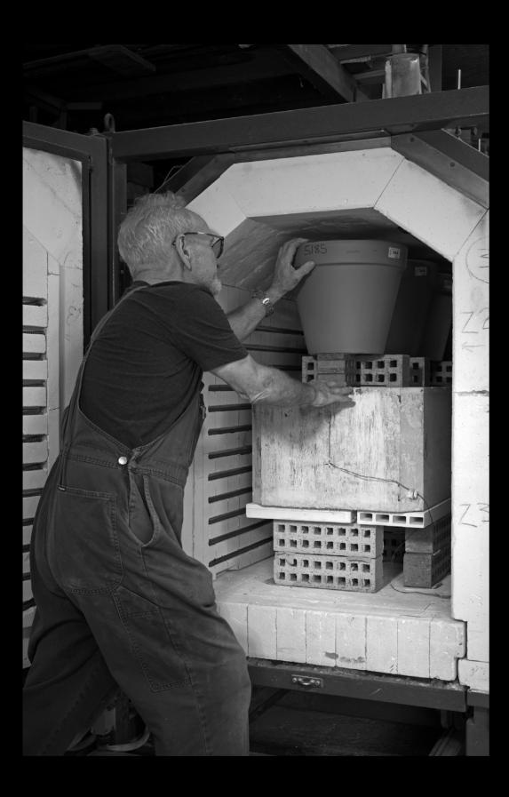
IMAGE / VESTIGE UNDERGOES A 28 DAY FIRING AND ANNEALING PROCESS
